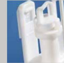
With one click the flushing volume can be changed from 6 to 7,5 litres, and back. This can be done without even having to remove the valve.
